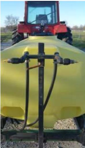
Last year, my sprayer pump lost pressure and I discovered that sprayer manufacturers install inexpensive pumps with plastic internal parts as a cost-saving measure. These pumps quickly break down if any sediment is present in spray mixtures. Our agricultural equipment dealer recommended purchasing a HYDRO commercial-grade pump at a cost of approximately \$375. If you are purchasing a new tank/pump or replacing an existing pump, be sure to buy a commercial grade pump such as the one shown below.
